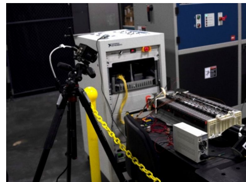
FLIR A70 thermal imaging camera monitoring battery pack tests.
