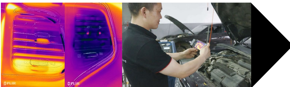
Possible leakage in air conditioning system. Normally working air conditioning system
